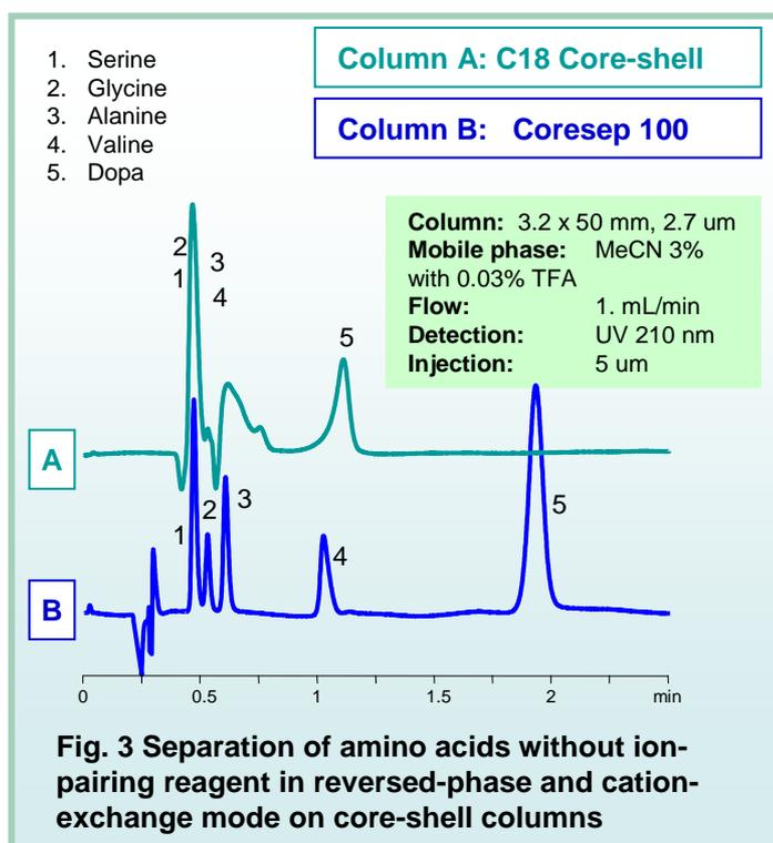
This low hydrophobicity and absence of ion-exchange mechanism prevents suitable retention in reversed-phase mode, but such amino acids can be effectively retained separated in reversed-phase cation-exchange using **Coresep™** columns. Five amino acids (SER, GLY, ALA, VAL and DOPA) were effectively retained and separated within 2 minutes.
