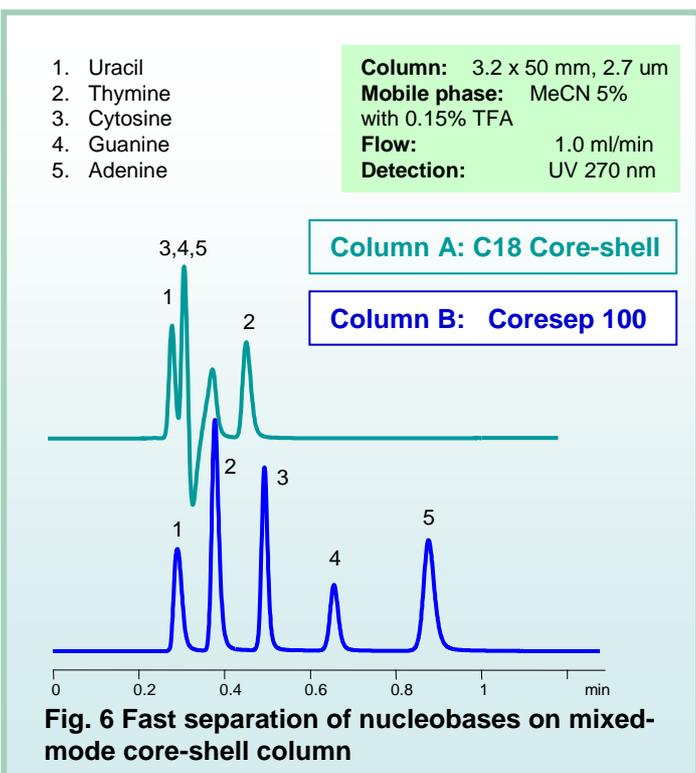
**Fast separation of Nucleobases on mixed-mode core-shell columns (Fig. 6)**
